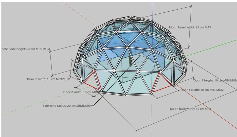
Fig 1. Clearances and dimensional specifications for space to fit the structure. These diagrams are a representation to show the **MINIMUM** interior dimensions of structures for the safe zone and **MAXIMUM** exterior dimensions of the Moon Base. Please note that the interior and exterior shape and placement of the openings of the Moon Base is to be determined by teams within the minimum and maximum requirements.
