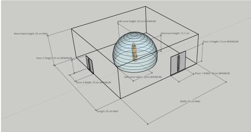
Fig 1. Clearances and dimensional specifications for space to fit the structure. These diagrams are a representation to show the MINIMUM interior dimensions of structures for the safe zone and MAXIMUM exterior dimensions of the Moon Base. Please note that the interior and exterior shape and placement of the openings of the Moon Base is to be determined by teams within the minimum and maximum requirements.
